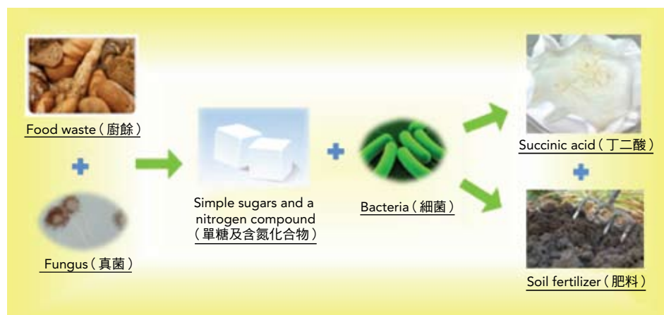
Figure 3. Schematic showing how food waste can be converted to succinic acid and fertilizer.
