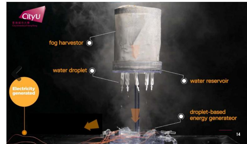
A network of the system can produce at least 100 litres of freshwater per day
