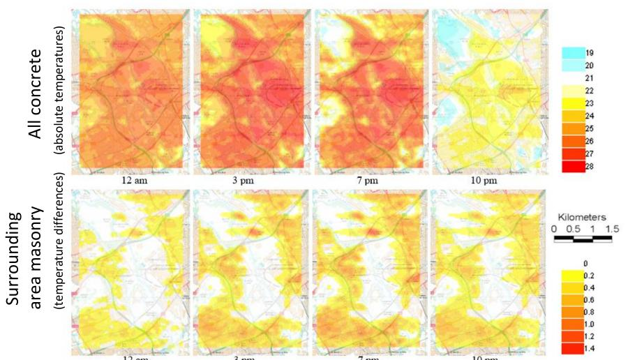
CONCRETE (high thermal admittance) vs MASONRY (low thermal admittance)
