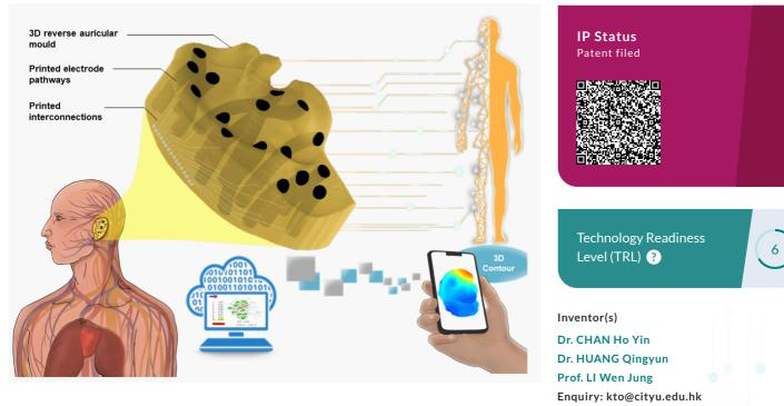
3D-printed personalized auricular sensor (3D-PAS) for simultaneously real-time bio-signal monitoring of multiple points across entire ear auricle.
