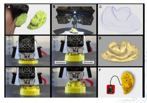
Fabrication process of 3D-PAS. (A) Human-specific auricular impression molding. (B) 3D-scanning of reverse auricular mold. (C) Points cloud generating. (D) Geometric designing and locating of embedded electrodes pathways. (E) 3D-printing of sensor with elastomer and functional material. (F) Prototype of
