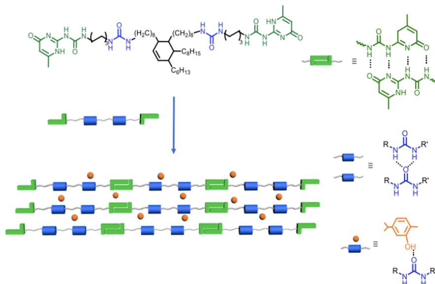
Scheme 1 Supramolecular organogels structure with long polymer chains and large-scale crosslinked network. Essential oil molecules tend to interact with carbonyl units by destroying weak hydrogen bond between urea-urea groups.
