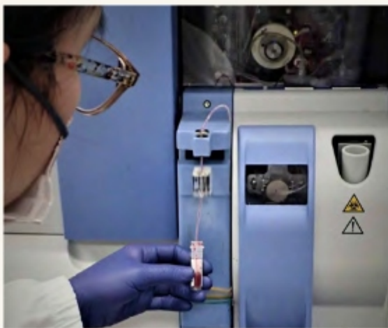
Figure 5: Cattle blood samples are loaded into the haematology analyser by a CityU VDL technologist for testing 圖5：城大動物醫療檢驗中心技術員將牛隻血液樣本載入血液學分析儀，以作檢測。
