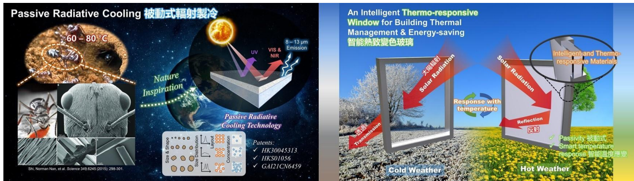
Figure 1: Smart and green building “skin” technology: passive radiative cooling and thermochromic smart windows
