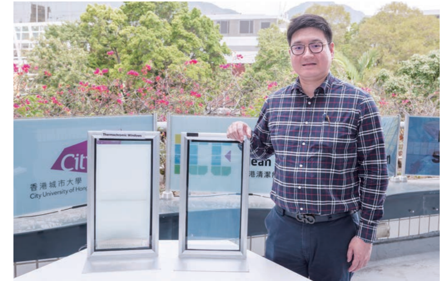
Prof. Edwin TSO and his team develop a reversible smart window with Near-Infrared-Activated Thermo-chromic Perovskite.
