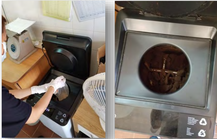
Mini food decomposer used in staff quarters for converting food waste into fertilizers
