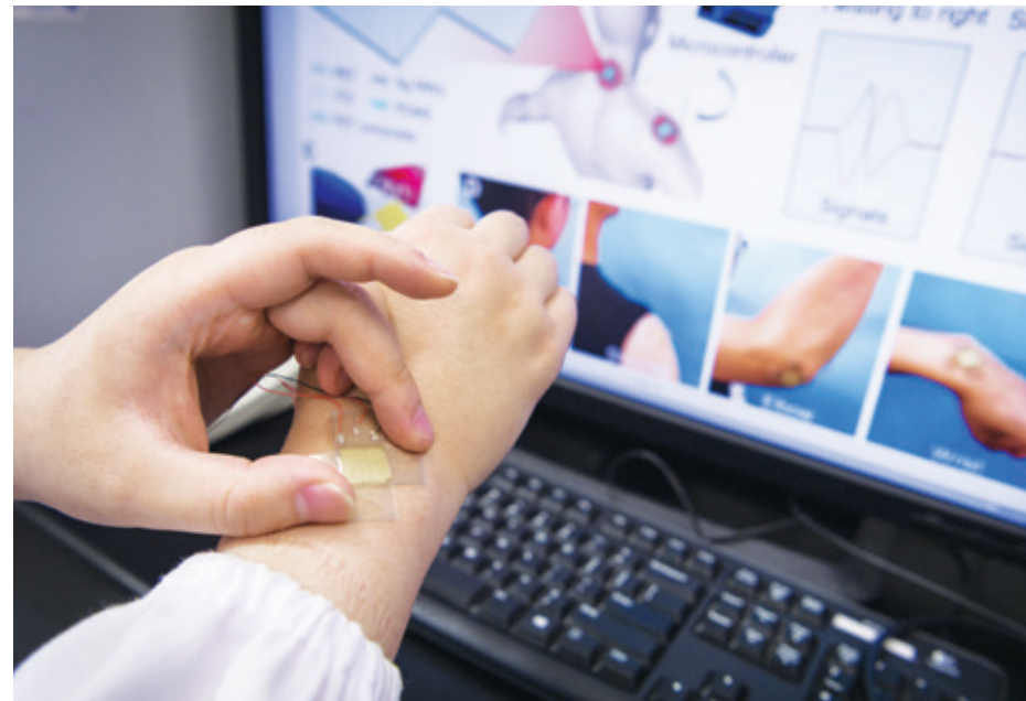
The kirigami-structure sensor that can monitor joint movements when attached to the body. 與人體連接後的剪紙結構傳感器能全面監測關節活動。
