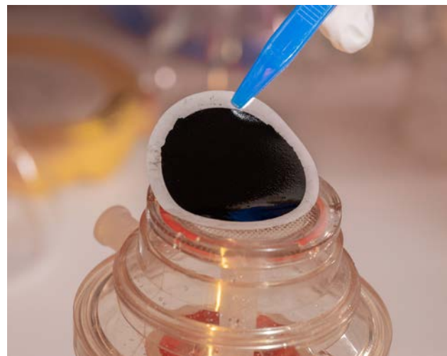
The membrane is coated with an ultrathin layer of MoS 2 , enabling it to capture DNA in water samples more effectively.
