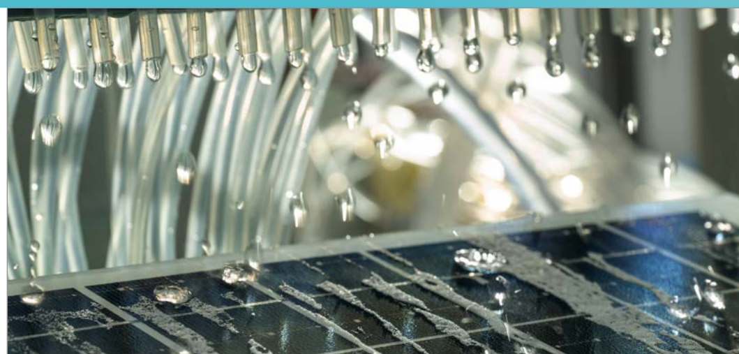
The innovative "Liquid Droplet Mop" technology precisely controls droplet impacts to effectively remove contaminants from solar panel surfaces.
