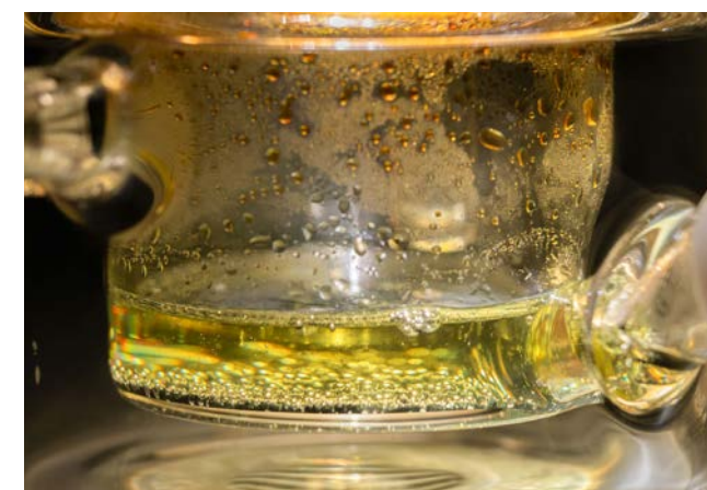
The system introduces copper ions to create a self-regenerating cycle, enabling continuous hydrogen production while recycling its own chemical waste.
