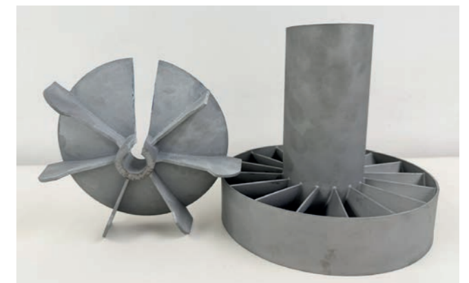
This photo shows components of power generation equipment produced using metal 3D printing technology.
