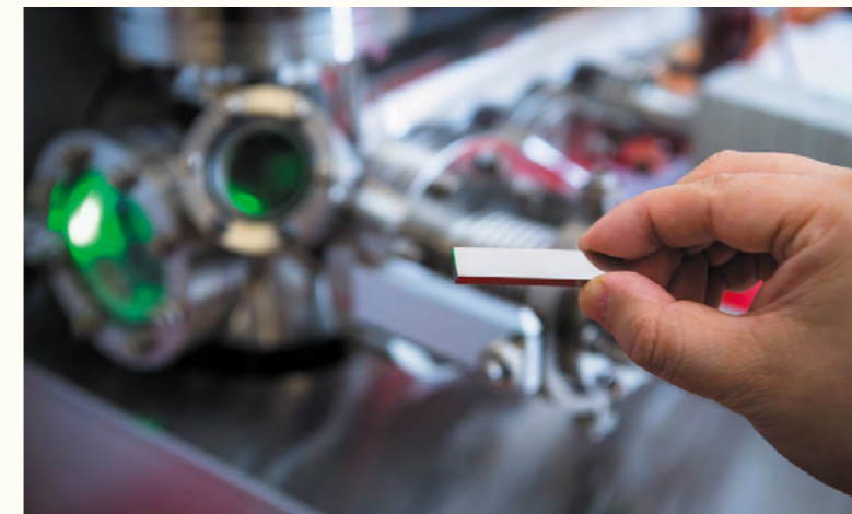
The stiffness of the the high-entropy Elinvar alloy remains invariant with temperature. (CityU) 研究發現高熵艾林瓦合金的剛度不會隨溫度而變化。
