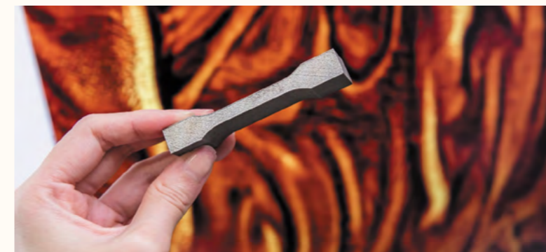
The titanium alloy developed by Professor Liu's team is super-strong, highly ductile and ultra-light [3]. 劉教授團隊開發的異質鈦合金非常堅固，且具有良好的延展性和較低的密度 [3]。
