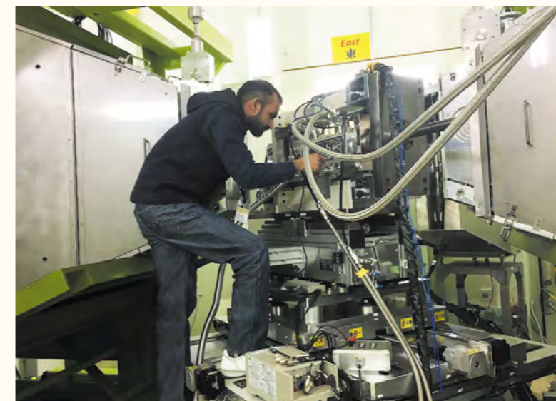
Muhammad NAEEM prepares the experiment at TAKUMI, an engineering materials diffractometer at Japan Proton Accelerator Research Complex (J-PARC) used to perform in-situ neutron diffraction measurements multiple HEA samples, which all showed a multi-stage deformation process.
