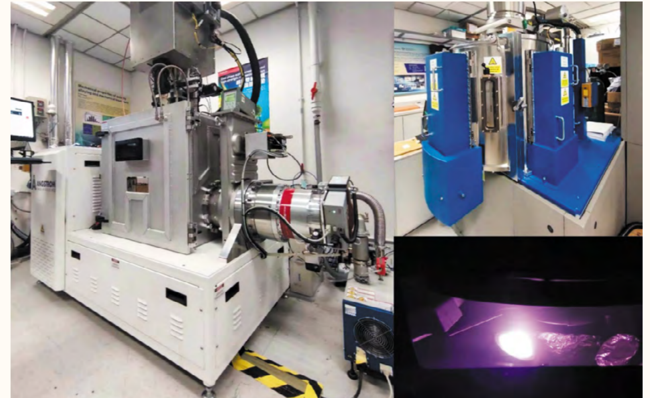
Figure 1 The advanced physical vapor deposition instruments at NPMM, introduced for the development of SNDP materials. 圖 1 NPMM 實驗室用於製備超納雙相納米材料的磁控濺射設備。
