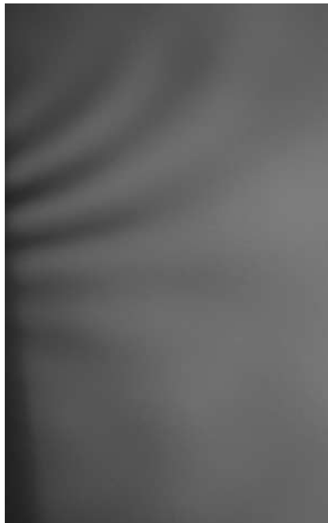
Fig. 21. Interference fringes produced using a radiochromic film.
