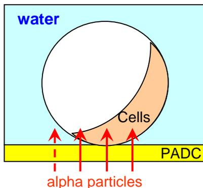
**Fig. 8.** Schematic diagram showing alpha-particle irradiation of a tilted zebrafish embryo. The alpha particle represented by the dashed arrow does not hit embryo cells and should therefore be discarded when calculating the radiation dose [16].
