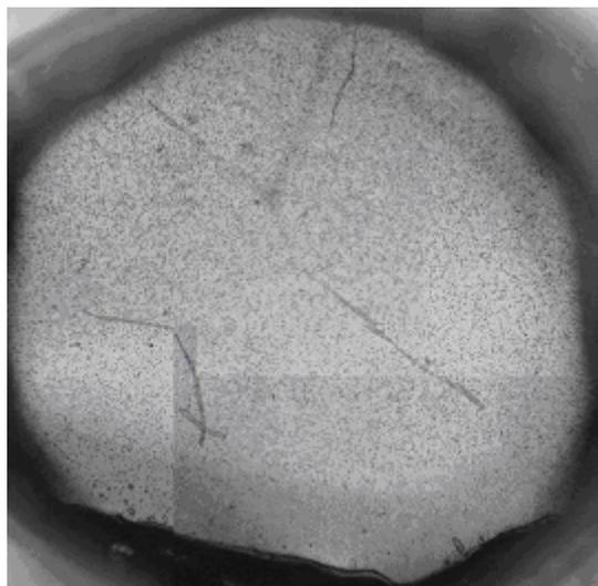
**Fig. 6.** An overall image of a PADc film at the bottom of the hole with visible alpha-particle tracks, reconstructed from 4 images covering different areas [16].
