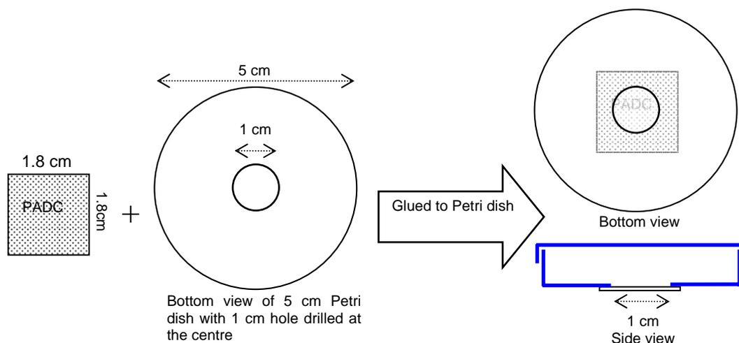
**Fig. 1.** Preparation of a custom-made PADC-film based holder by gluing a thin PADC film onto the bottom of a petri dish with 5 cm diameter and with a 1 cm hole drilled at the center of the bottom.
