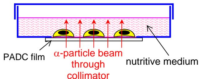
**Fig. 2.** The irradiation of the cell monolayer through the custom made PADC cell dish.
