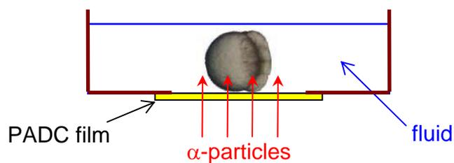
**Fig. 5.** Schematic diagram showing alpha-particle irradiation of a zebrafish embryo at 1.5 hpf, with the yolk and one layer of cells touching the support substrate, and assuming that the alpha particles strike the PADC film vertically.
