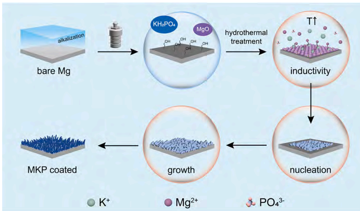
Fig. 12. Schematic diagram of the MKP coating formation process.
