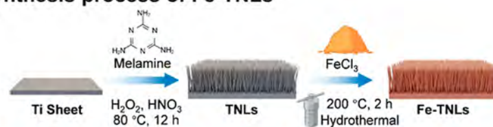
Scheme 1. Schematic Illustration of the Preparation of Fe-Doped Titanium Dioxide Nanolines for Sustainable Wastewater Sterilization with Electrically Stimulated Regeneration of POD-like Activity a
