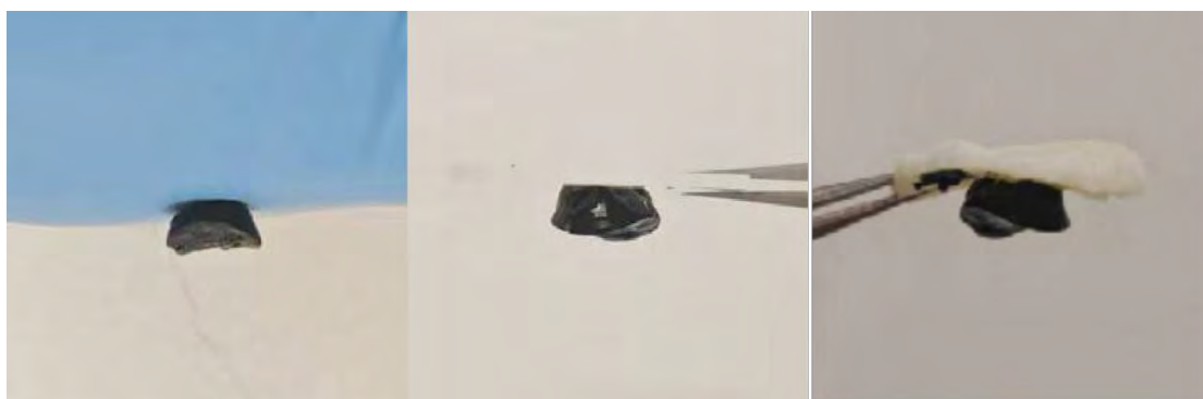
Figure S4. Adhesive performance evaluation of AT-PP@MnO 2 on nitrile gloves (left), glass (middle), and porcine skin (right).
