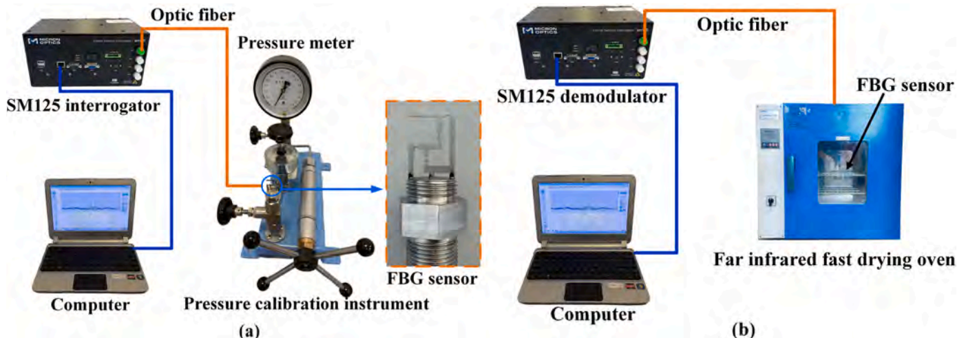
Fig. 5. Test systems: (a) pressure testing; (b) temperature testing.
