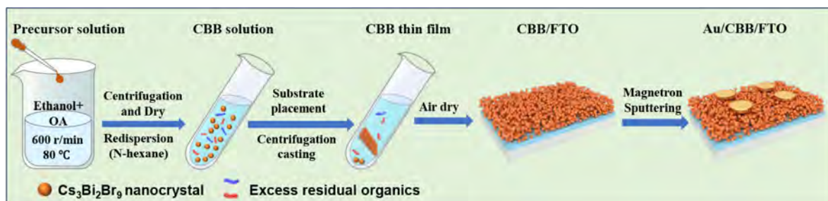
Scheme 1. Schematic of the Synthesis of the Au/CBB/FTO Devices
