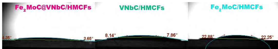
Fig. S3. Water contact angles on \text{Fe}_2\text{MoC@VNbC/HMCFs} , \text{VNbC/HMCFs} , and \text{Fe}_2\text{MoC/HMCFs} .
