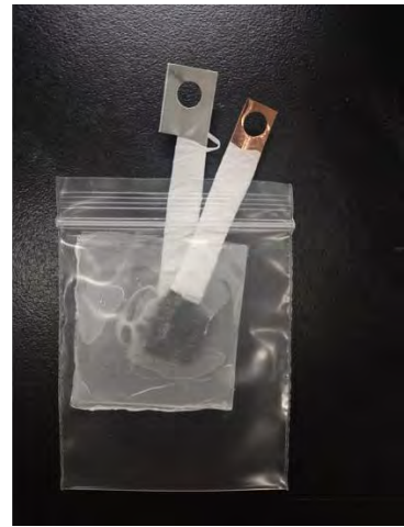
Fig. S1 Schematic and photograph of flexible Ni-Zn battery.
