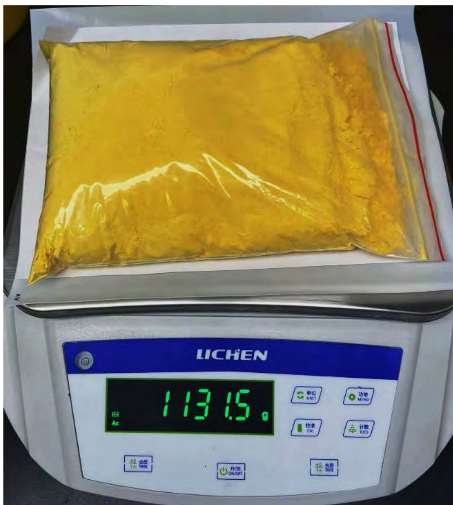
Figure S1. CsPbBr 3 powder synthesized by mechanical grinding.
