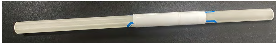
Fig. 14. Photograph of connected notch Bar-THz HC-ARF.
