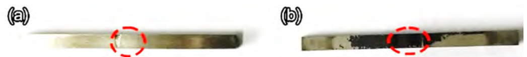
Figure 9. Photographs of (a) S4 and (b) S9 immersed in the acidic NaCl solution for 30 days.
