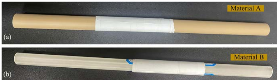
Fig. 11 Photographs of the connected waveguides
