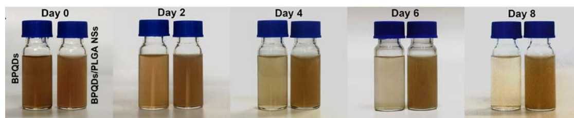
Figure 2. Photographs of the BPQDs and BPQDs/PLGA NSs after storing in water for different periods of time.
