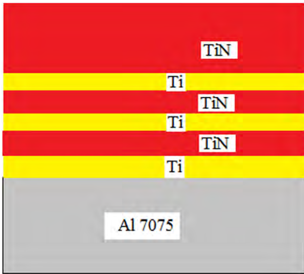
Fig. 1. Structure of the Ti/TiN multilayered coating on Al 7075.
