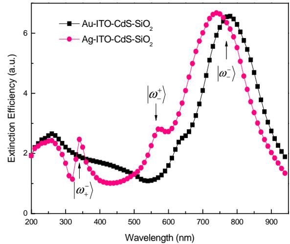
Fig. 5. Comparison of the extinction spectra: Au-ITO-CdS-SiO<sub>2</sub> and Ag-ITO-CdS-SiO<sub>2</sub> multilayered nanoshells as a function of refractive index of the surrounding medium.
