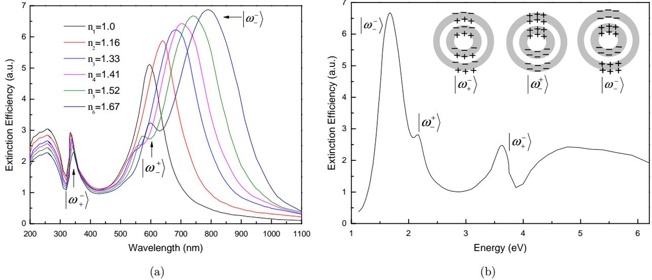
Fig. 2. (a) Extinction spectra of the Ag-ITO-CdS-SiO<sub>2</sub> multilayered nanostructure as a function of refractive index of the surrounding medium; (b) Extinction spectra of the three types of plasmonic coupling modes based on the LSPR of the Ag-ITO-CdS-SiO<sub>2</sub> multilayered nanostructure.
