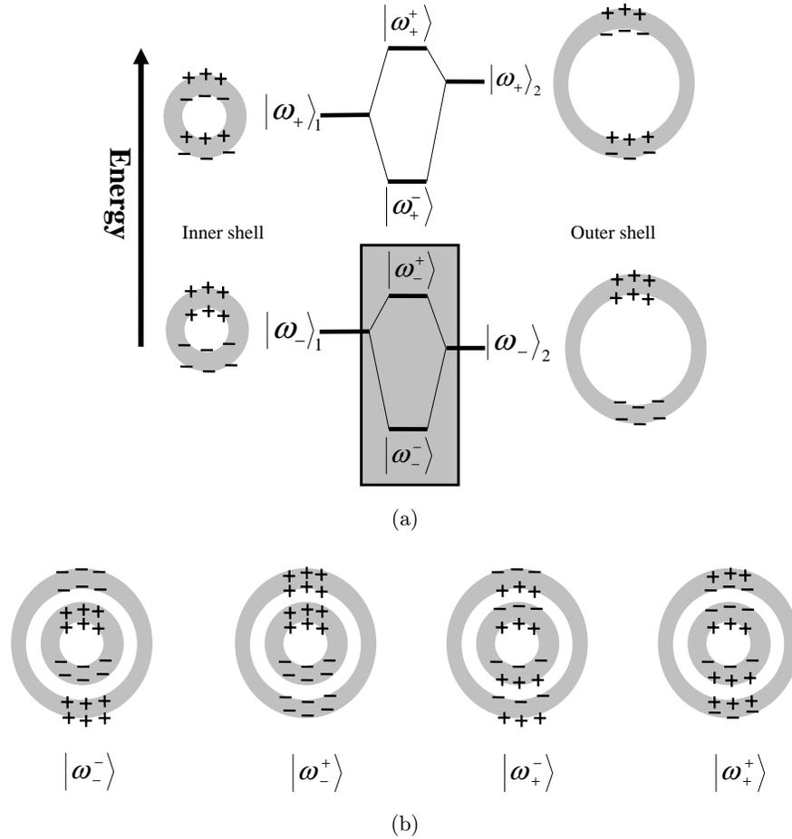
Fig. 3. (a) Energy level diagram of the plasmon modes of multilayered nanoshell; (b) Induced polarizations of the concentric nanoshell modes.
