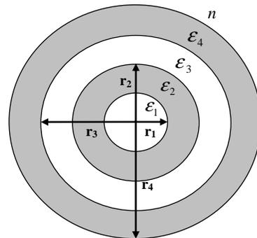
Fig. 1. Schematic representation of the concentric multilayered nanosphere.
