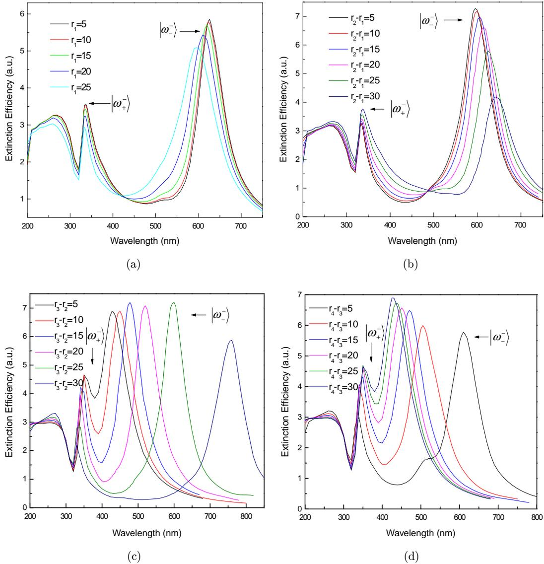
Fig. 6. Calculated extinction spectra of Ag–ITO–CdS–SiO<sub>2</sub> multilayered nanoshells as a function of refractive index of the surrounding medium with different (a) SiO<sub>2</sub> core thickness; (b) CdS inner shell thickness; (c) ITO middle shell thickness; and (d) silver outer shell thickness.
