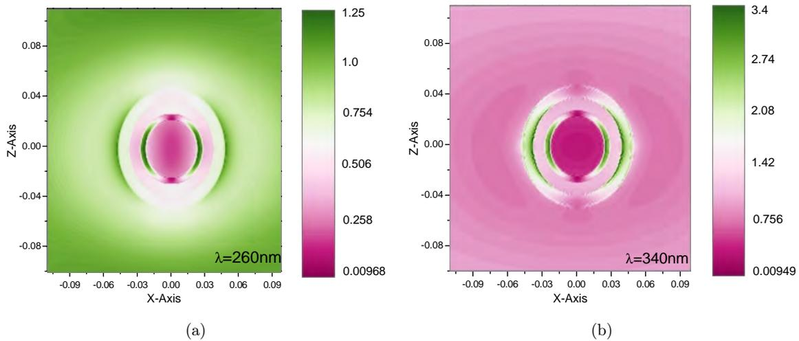
Fig. 4. Electric field enhancement contour around Ag-ITO-CdS-SiO<sub>2</sub> multilayered nanostructure under illumination at plasmon resonance wavelength.
