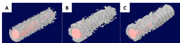
Fig. 2. Reconstructed three-dimensional images of bone on implant surface: (A) untreated Ti; (B) carbon-PIII treated Ti and (C) nitrogen-PIII treated Ti
