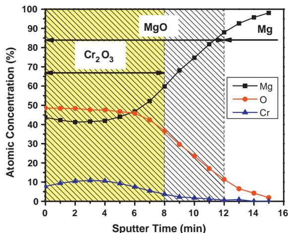
Fig. 1. XPS depth profiles of the implanted sample.
