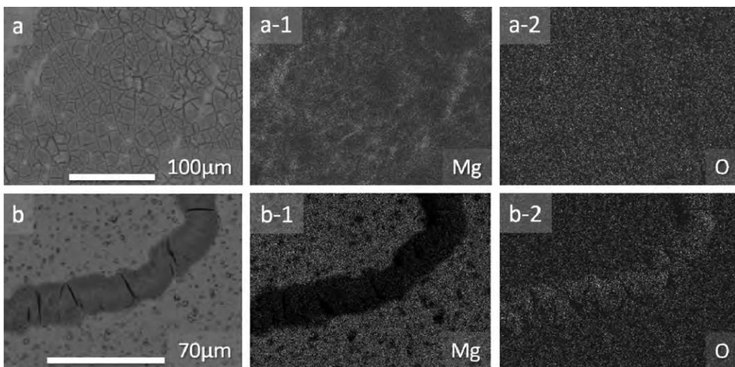
**Fig. 8.** Elemental maps of Mg and O on different samples after immersion in SBF: (i) SEM images, (i-1) Mg elemental maps, and (i-2) O elemental maps [i = a and b denoting pure Mg and implanted sample].
