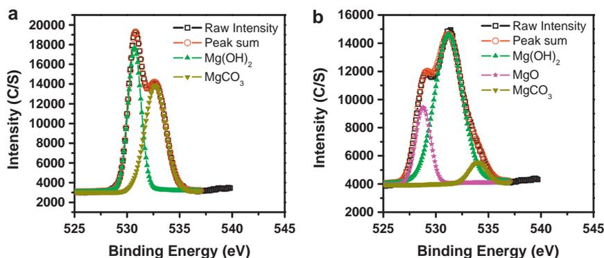
**Fig. 6.** Fitted curves of the O 1s XPS spectra obtained from Mg after immersion in  $\text{Na}_2\text{SO}_4$  solution: (a) surface and (b) at a depth of 50 nm.
