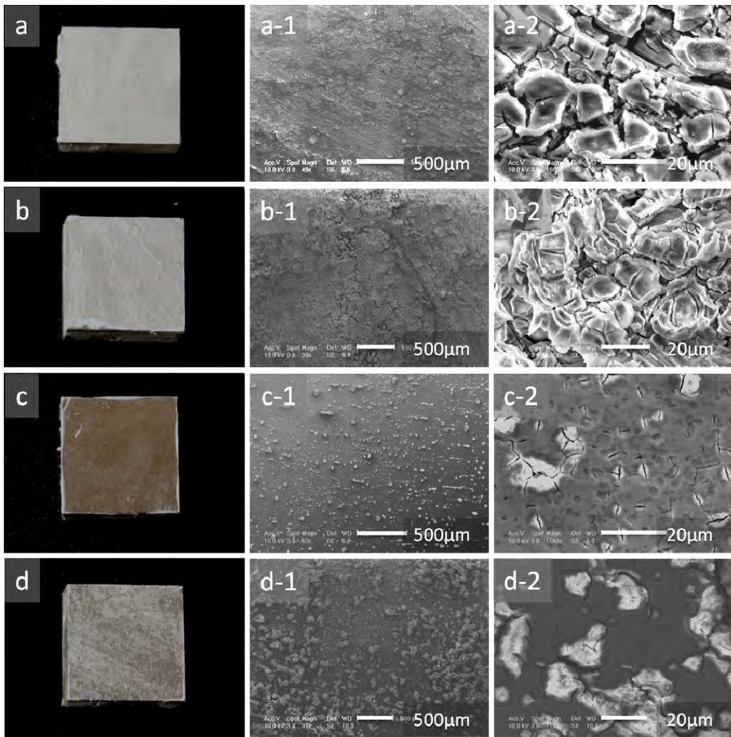
**Fig. 7.** Morphological images of different samples immersed into SBF: (i) digital camera pictures, (i-1) low-magnification SEM pictures, and (i-2) medium-magnification SEM pictures [i = a, b, c, and d denoting Mg-3h, Mg-18, implanted-3h, and implanted-18h].
