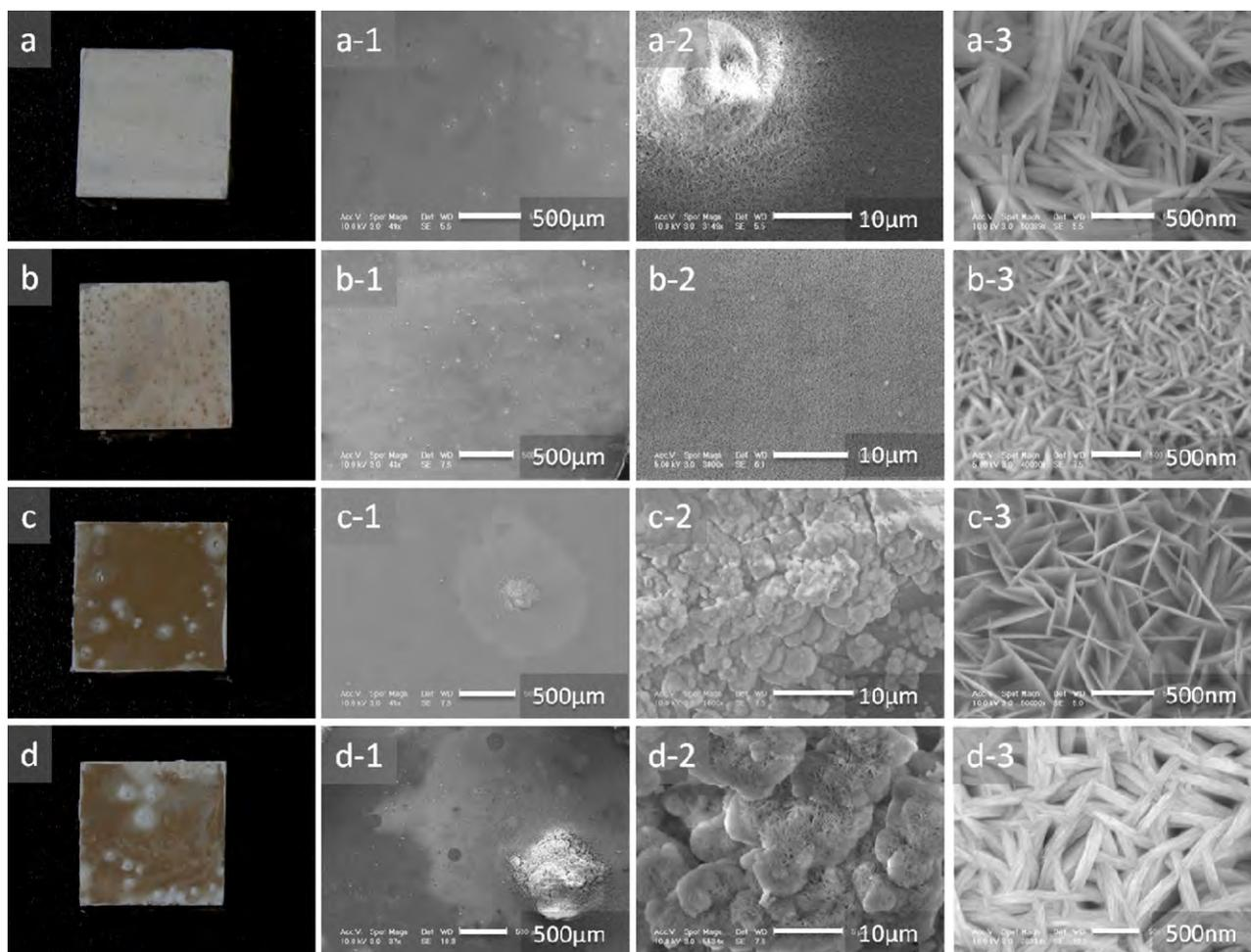
**Fig. 5.** Morphological images of different samples immersed into  $\text{Na}_2\text{SO}_4$  solution: (i) digital camera pictures, (i-1) low-magnification SEM pictures and (i-2) medium-magnification SEM pictures, and (i-3) high-magnification SEM [i = a, b, c, and d denoting Mg-3h, Mg-18, implanted-3h, and implanted-18h].
