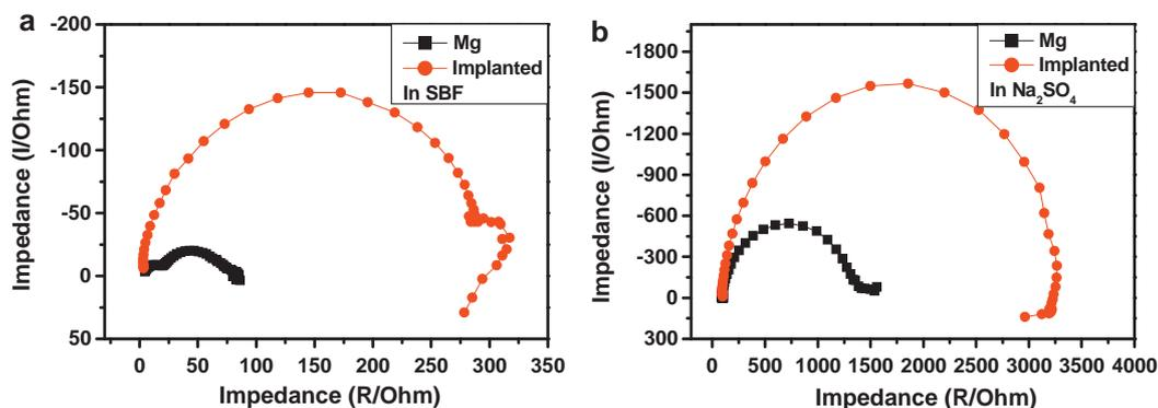
Fig. 4. Typical electrochemical impedance spectra of Mg and implanted samples immersed in (a) SBF and (b)  $\text{Na}_2\text{SO}_4$  solution.
