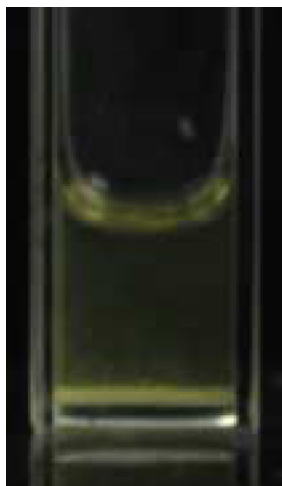
Fig. 1. Optical image of the newly-prepared water suspension of 3C-SiC nanocrystallites with illumination of room light by using fluorescent lamps.
