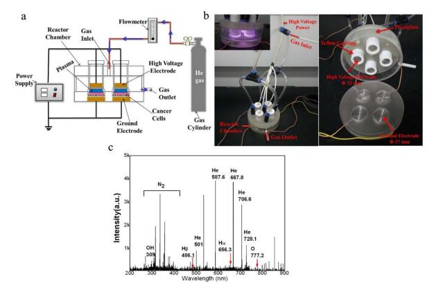
**Figure 1.** Schematic of the non-thermal plasma device. (a) Schematic of the plasma system. (b) Photographs of reactor chamber. (c) Typical optical spectrum of helium plasma.
