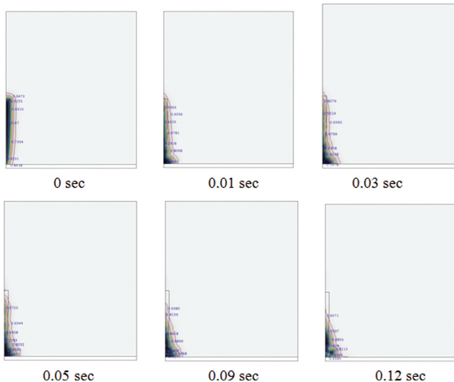
FIG. 14. Distribution of volume fraction of carrier gas in grid 1.
