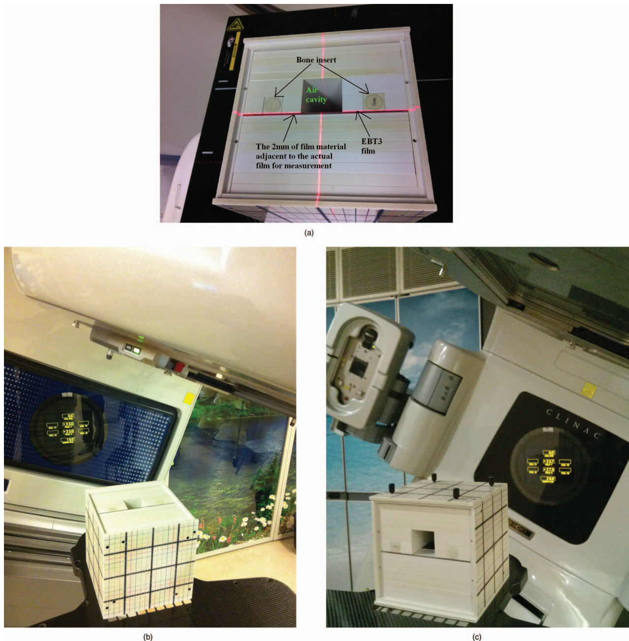
FIG. 1. The (a) coronal view of head and neck cube of the Scanditronix Wellhofer I mRT phantom containing air cavity and bone insert, and its position relative to the radiation beam during measurement of planar dose distribution on (b) axial plane and (c) coronal plane.
