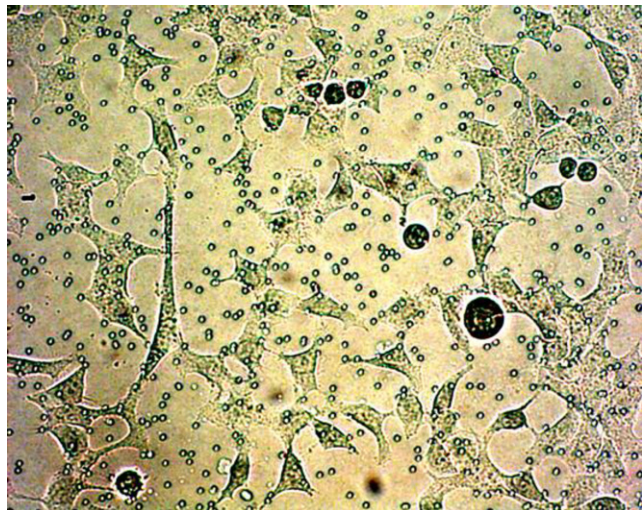
Fig. 3. An image (200 \times in the transmission mode) showing the superposition of HeLa cells cultured for 3 d and track-etch pits generated from irradiation of 3 MeV alpha particles for 3 h, etched for 3 h in 6.25 N aqueous NaOH at 70 ^{\circ} C and then for 5 min in 1 N NaOH/ethanol at 40 ^{\circ} C.
