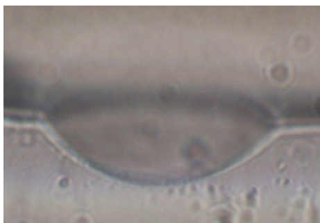
Fig. 2. The lateral view of a spherical track (from an alpha particle with incident energy of 3 MeV and pre-etched in 6.25 N NaOH/water at 70 °C for 4 h and then further etched in 1 N NaOH/ethanol for 15 min) revealed under the optical microscope operated in the transmission mode after polishing the edge of the detectors.
