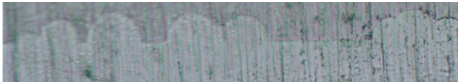
Figure 3. Optical microscopic image showing the cross sections of the tracks with the dried replicating fluid inside. The upper part is the detector while the lower part is the replicating fluid. The replicas of the tracks are shown clearly.
