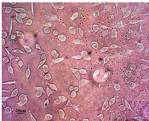
Figure 3. The image of the HeLa cell monolayer on a thin PADc film with revealed alpha-particle tracks under the optical microscope with a magnification of 200 \times (taken from the side of the cell monolayer). The 5 MeV alpha-particle tracks are seen on the right hand side as black dots. These tracks are developed on the underside of the PADc film (which is glued to the bottom of the cell dish) after chemical etching in (while floating on) a 14 N KOH solution at 37 ^{\circ} C for 4 h. (Adopted from Chan et al. 2007a.)
