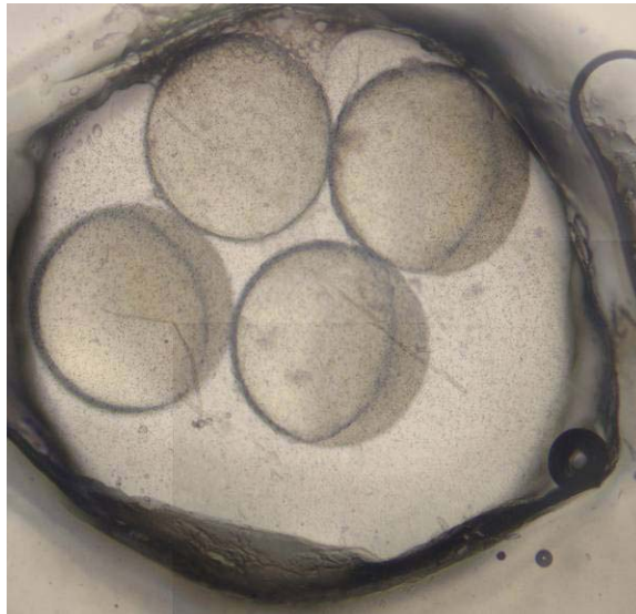
Figure 11. Superposition of (a) the image of the PADc film at the bottom of the hole with visible alpha-particle tracks shown in Figure 10 with (b) the image of embryos. (Adopted from Yum et al. 2007.)
