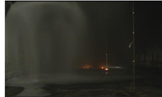
(d) Fire extinguished at 10 s after activating WFFF system
