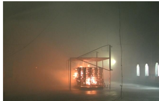
(f) 300 s after activating WFFF system
