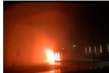
(e) 180 s after activating WFFF system
