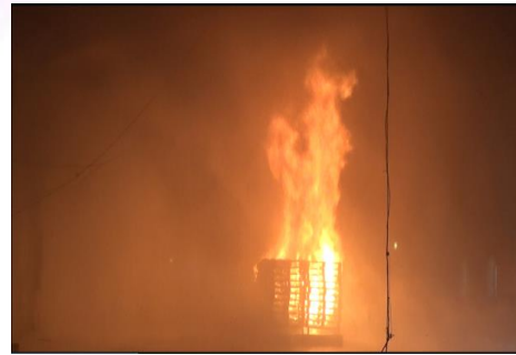
(b) 60 s after activating WFFF system
