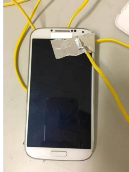
(b) Thermocouples at different components
