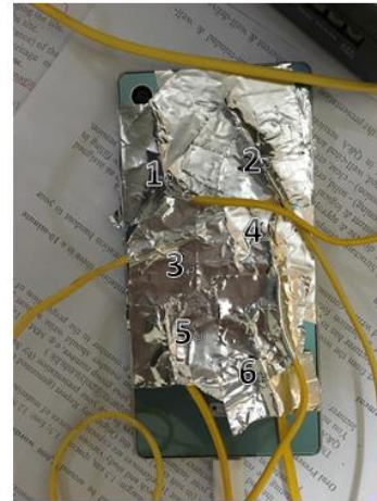
(b) Cover removed to see thermocouples at different components
