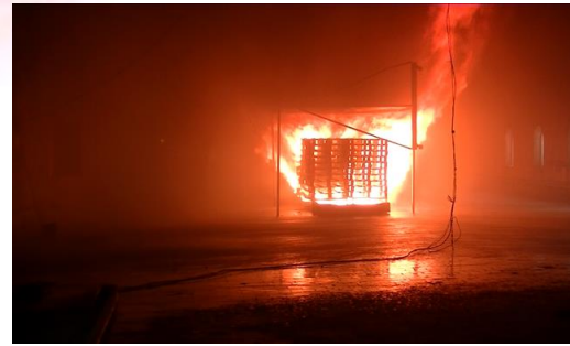
(b) 60 s after activating WFFF system
