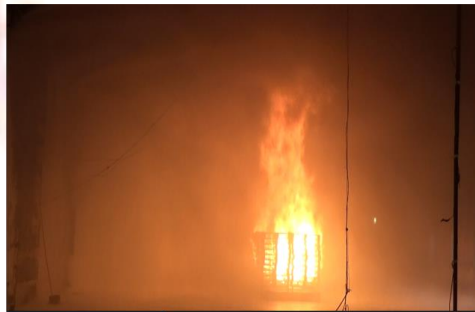
(c) 120 s after activating WFFF system
