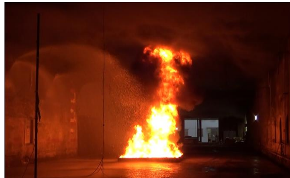
(b) WFFF system activated
