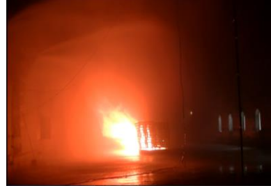
(c) 60 s after activating WFFF system
