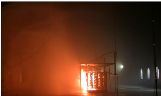
(e) 180 s after activating WFFF system
