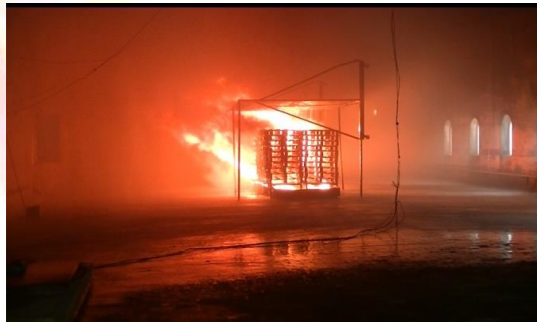
(c) Ventilation system activated at 90 s
