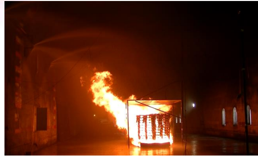
(b) WFFF system activated
