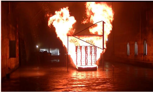
(a) Wood pallet burning with the top shield
