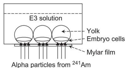
Figure 1. Irradiation of 5 hpf zebrafish embryos with alpha particles through a Mylar film-based holder.
