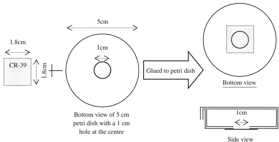
Fig. 1. Preparation of a custom-made PADC-film based holder by gluing a thin PADC film onto the bottom of a petri dish with 5 cm diameter and with a 1 cm hole drilled at the center of the bottom (Chan et al., 2006).
