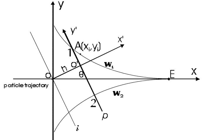
Fig. 1. Construction of an alpha-particle track in the detector. The particle trajectory is along the  $x$ -axis. The entrance point  $O$  is chosen as the origin of the coordinate system and  $E$  is the end of trajectory, so  $OE = R$  (range). The initial and post-etching detector surfaces are represented by  $i$  and  $p$ , respectively. The curves  $w_1$  and  $w_2$  represent the loci of the particle track in the cross section ( $z=0$ ).
