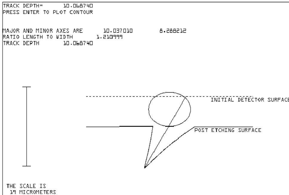
Fig. 2. The track profile and track-opening contour obtained for the CR-39 detector, for the input parameters as stated in the text.
